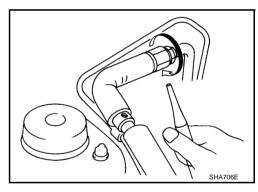
3. Move probe along component approximately 25 to 50 mm (1 to 2 in)/sec.
