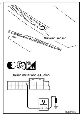
• When checking sunload sensor, select a place where sunshine directly on it.
