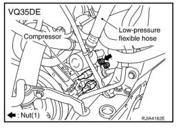
8. Remove mounting nuts from low-pressure flexible hose and low-pressure pipe (VK45DE).
