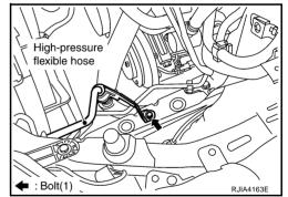
3. Remove high-pressure pipe 1 from vehicle clips.
