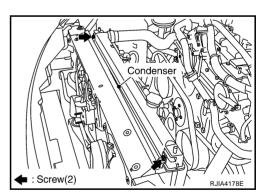
16. Pull condenser forward at an angle. Remove condenser from radiator.
