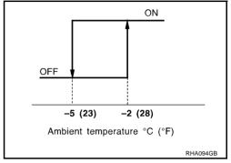
When intake air temperature is higher than  $1^{\circ}$ C ( $34^{\circ}$ F), the compressor turns ON. The compressor turns OFF when intake air temperature is lower than  $-5^{\circ}$ C ( $23^{\circ}$ F).
