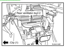
3. Remove mounting clips, and then remove rear ventilator ducts
