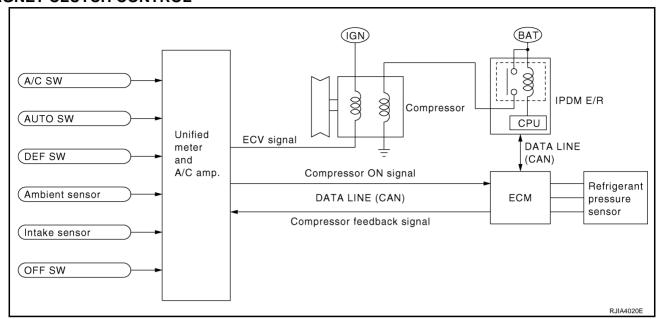
When A/C switch, AUTO switch or DEF switch is pressed, unified meter and A/C amp. transmits compressor ON signal to ECM, via CAN communication.
