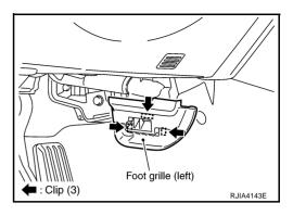
Remove mounting clips, and then remove foot grille (right).
